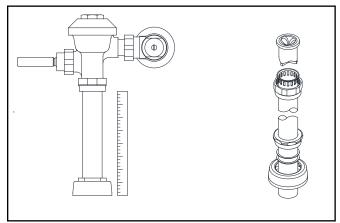
**5.** Hand tighten spud nut and vacuum breaker tube nut to fixture and flush valve. Adjust the valve assembly for plumb. Tighten fixture spud nut, vacuum breaker tube nut and lock nut with a wrench.
