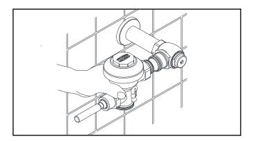
Insert the flush valve tailpiece into the stop valve and hand tighten the lock nut to the stop valve. Plumb the entire unit (see 3).
