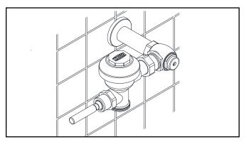
4. Determine the length of vacuum breaker tube required to join the flush valve and fixture spud. Cut the vacuum breaker tube, if re quired, to this length (see 4a). Assemble the vacuum breaker tube assembly and spud nut assembly to the flush valve and fixture spud (see 4b).
