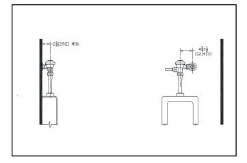
Models: Z6001AV (1-1/4" urinal flush valve) Z6003AV (3/4" urinal flush valve)
