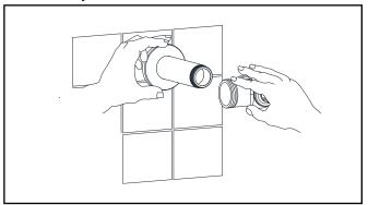
2. Prior to inserting the flush valve tailpiece into stop valve, be certain that the O-ring seal is located in O-ring seal groove at the end of the tailpiece and the locking nut and locking snap ring are located as shown below (see 2). Care should be taken not to damage the O-ring when inserting the tailpiece into the stop valve. If lubrication is needed, wetting the O-ring with water will be sufficient.
