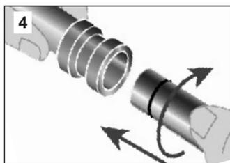
4. Holding the fitting tightly, insert the tube straight into the fitting with a twisting motion, as shown, until the depth mark on the tube outside diameter is aligned with the end of the fitting. If the mark and the end of the fitting are not aligned, then continue to push the tube to the full insertion depth. A gentle pull will indicate if the connection has been properly made. Absolutely NO lateral movement should occur! Any lateral movement could indicate an improper insertion depth
