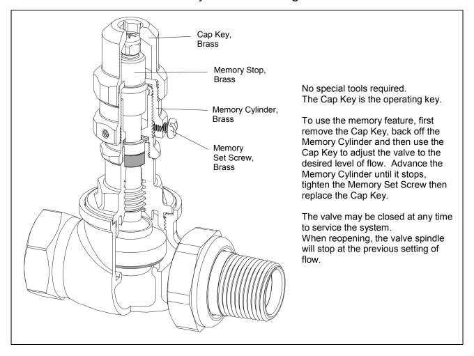
Design Features: Same as #13000 balancing valve (see TDS-1007) except for the "memory" components shown above.
