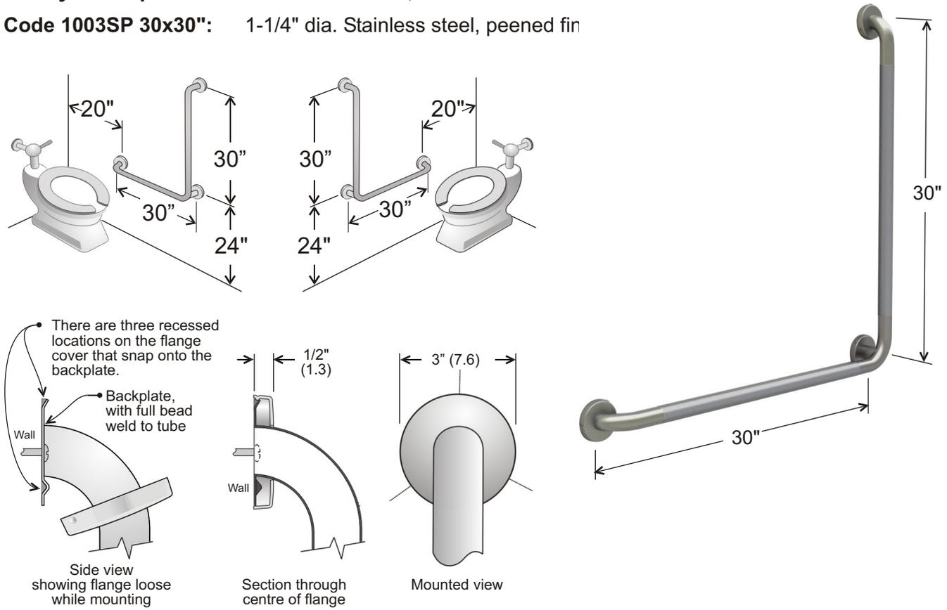
Concealed mounting screws, using snap flange, on "SP & NP" codes
