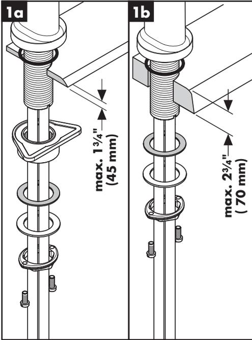
Place the faucet and sealing ring on the mounting surface.
