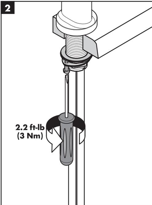
Tighten the mounting nut.
