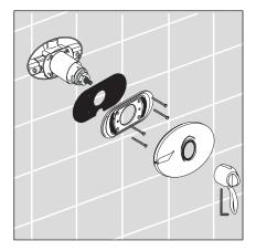
Use a 3 mm Allen wrench to loosen the set screw on the handle.
