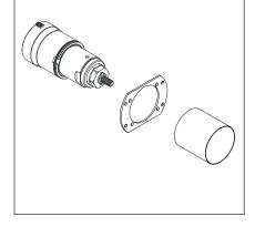
Install the new thermoelement on the valve.
