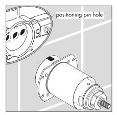
Install the cartridge. To prevent damage to the cartridge, make sure that the positioning pin goes straight into the hole.
