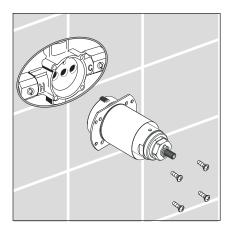
Remove the sleeve and retainer plate from the old element. Carefully install them on the new thermoelement.
