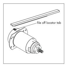
Older TP/TB I roughs have only the hole for the positioning pin – they do not have a notch for the locator tab. If you have an older rough, carefully file the black plastic locator tab off of the new cartridge. Be careful not to damage the cartridge.
