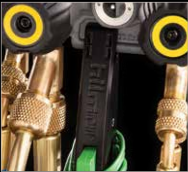
Attach K-style clamp to an easily accessible spot on the hilmor manifold.
