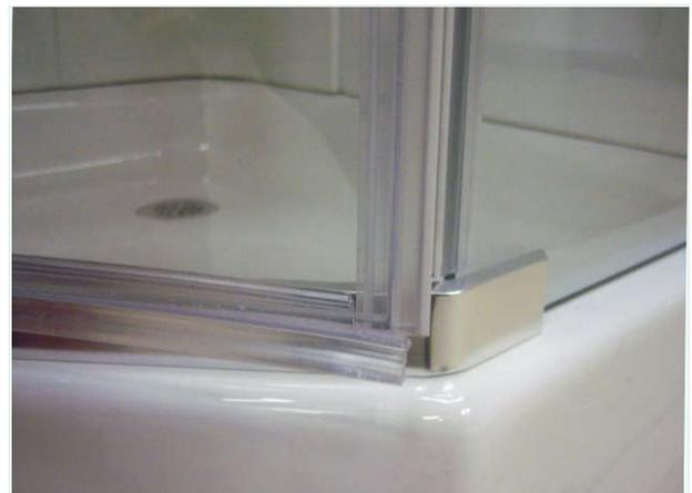
STEP 31: Top and bottom of the Door Panel (8) can be adjusted to improve the magnet seal when closing the door. Loosen the steel nuts (5J) and move the Door Panel (8) left and right.
