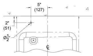
2. Drill 1/2" dia. hole thru drinking fountain deck (where shown above). Deburr hole and install grommet provided.
