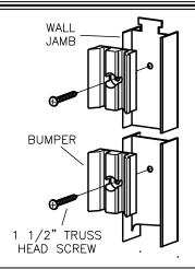
This bath enclosure is equipped with safety teelock wall jambs. When installed properly, the header is permanently locked to the wall jambs and cannot be accidentally dislodged.
