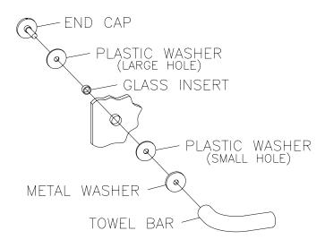
Insert the wrench [Q] into the small hole on the edge of an end cap [I] and rotate in a clockwise direction until tight. Repeat for all remaining end caps.
