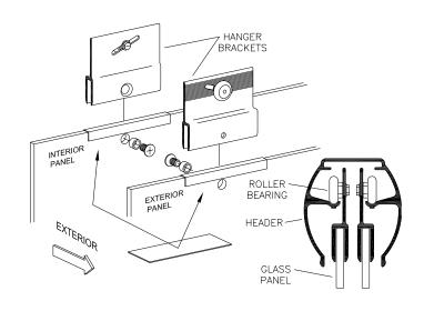
**CAUTION** – Do not over tighten the brackets and cause the attach the roller to the hanger bracket should be torqued to end to clamp down on patterned glass. Do NOT use a screw
