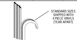
Cut four pieces of the smaller vinyl [HH] 1" longer than the vertical opening (to prevent gapping from shrinkage) and trim the ends on a 45° angle. Using the masking tape guides, center the glass panel [F] in the frame. Cut four short (1" - 2") pieces of the small vinyl and press into the jamb and post on each side to hold the glass temporarily.
