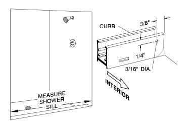
Place the two wall jambs [B] into the ends of the curb [A]. Masking tape may be used to hold the curb in place during this operation. Plumb the jambs and mark the hole locations on the wall. Remove all parts and drill the walls for mounting hardware.
