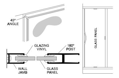
Cut four pieces of the larger vinyl [JJ] 1/2" longer than the horizontal opening and trim the ends on a 45° angle. Install the top exterior vinyl starting at both ends and working toward the middle. Be careful not to stretch the vinyl.
