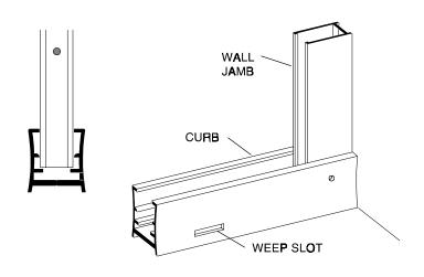
Wipe the shower walls and sill, the curb [A] and the wall jambs [B] with a clean, dry cloth to remove any dust or debris. Apply a 1/4" bead of caulk along the inside of both of the pencil lines marked in Step #2. Carefully replace the curb in the exact position marked. Caulk the inside of the curb ends where they meet the wall.
