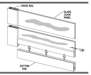
Press the hinge jamb/door panel assembly [\*A] and strike jamb [\*B] (with magnetic strip) over the wall jamb and/or framing posts. Refer to Step #1 of the STIKSTALL instruction sheet for the proper handing of the door.
