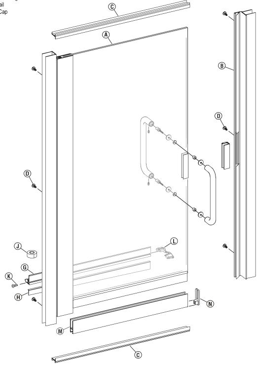
NOTE: Obscure glass doors should be installed with the rough surface of the glass to the exterior of the unit. Silk Screened or etched glass doors should be installed with the patterned surface to the inside.
