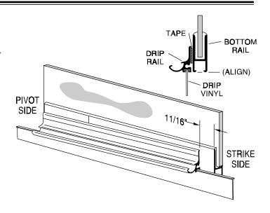
Adjust the drip vinyl [U] by sliding it left or right until it just touches the curb. Trim the vinyl (flush with the pivot end and notch 1/2" longer than the drip rail as shown on the strike end). Secure it with one #6 x 3/8" truss head screw [EE] in the pivot end of the drip rail [S].
