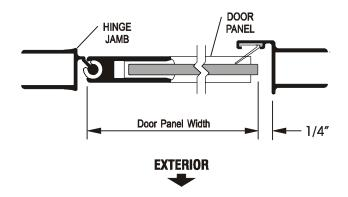
Snap both fillers [\*C] into the curb and header between the hinge and strike jambs with the raised lips to the exterior. Center the curb filler between the hinge and strike jamb (use masking tape to hold in position).
