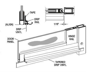
Adjust the drip vinyl [\*H] by sliding it left or right until it just touches the curb. Trim the vinyl flush with the hinge side and notch 1/2" longer than the drip rail [\*G] as shown on the strike side. Slide the vinyl into the drip rail and secure it on the hinge side of the drip rail with one #6 x 3/8" truss head screw [\*K].
