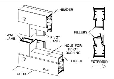
Pull the bottom end of the pivot jamb [L] tight to the curb filler [N] and plumb the jamb. Drill two 1/8" holes thru the pivot jamb and into the wall jamb [B] 3/8" to 3/4" from the wall and approximately 1/4" from the ends of the jamb. Drill a third hole centered between the first two, then enlarge the three outer holes with a 3/16" drill for clearance on the self-tapping screws. Attach the pivot jamb permanently with three #8 x 1/4" truss head screws [J].
