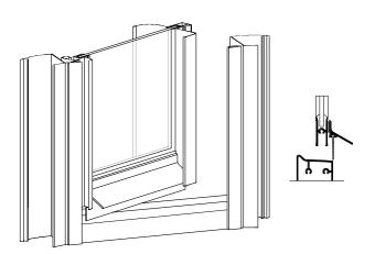
Wipe the shower walls and sill, and shower door assembly with a clean, dry cloth to remove any dust or debris. Apply a 1/4" bead of silicone along the inside and outside of both wall jambs at the wall surface, and along the outside of the curb at the shower sill surface, but not inside along the bottom of the curb, to allow any water that gets into the extrusion to drain back into the shower.
