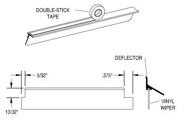
6 Hold the drip deflector [**D**] against the inside of the door bottom rail, positioning it properly so that the door closes without interference. Mark the location of the drip deflector on the top edge and side. Peel the backing off of the double stick tape [**K**] and carefully (you only get one try) stick the drip deflector to the door using the marks for alignment.
