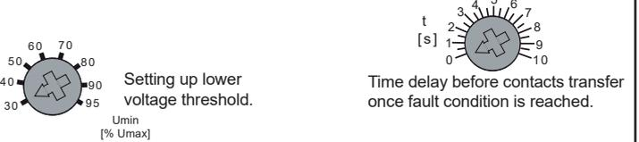
Once monitored voltage reaches the Umin, the time delay is initiated. After time delay is complete, the contacts 15-18 open and only red LED is ON.
