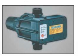
**Mascontrol**\* - Eliminates the pressure tank and switch from a conventional pump setup. It allows the pump to maintain a constant pressure and flow. Mascontrol can be used with either surface or submersible pumps. It also features a built in check valve, run dry protection, dual voltage wiring in either 115V or 230V.
