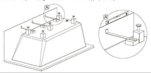
Ensure the apron is fixed firmly with the bathtub's bottom, then adjust the feet to make bathtub level to finish the installation. **Note**: *If you use the preleveled feet, this step is not neccessary.*
