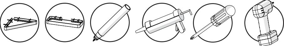
A. Place the metal frame of the shelf in the desired position. Level and mark the position of the holes.
