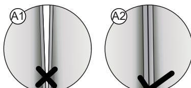
⚠ Adjust the sliding doors using the screws located on the bottom of top roller assemblies. Adjust rollers so that the sliding doors are parallel to the fixed panels and parallel to each other.
