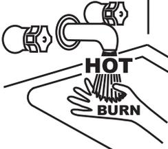
Water temperature over 125°F (52°C) can cause severe burns instantly resulting in severe injury or death.
