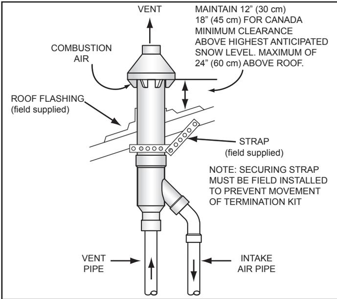
**Figure 29. Concentric Termination Clearances - Vertical Installation**
