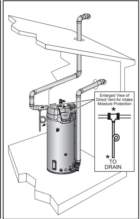
Figure 47. Direct Vent Horizontal Vent Vertical Intake
