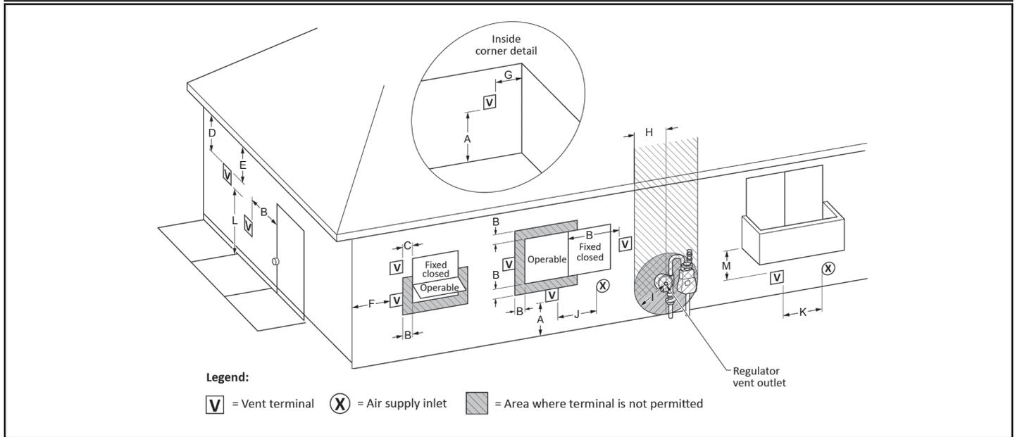
**Figure 52. Sidewall Direct Vent Using Outside Air**
