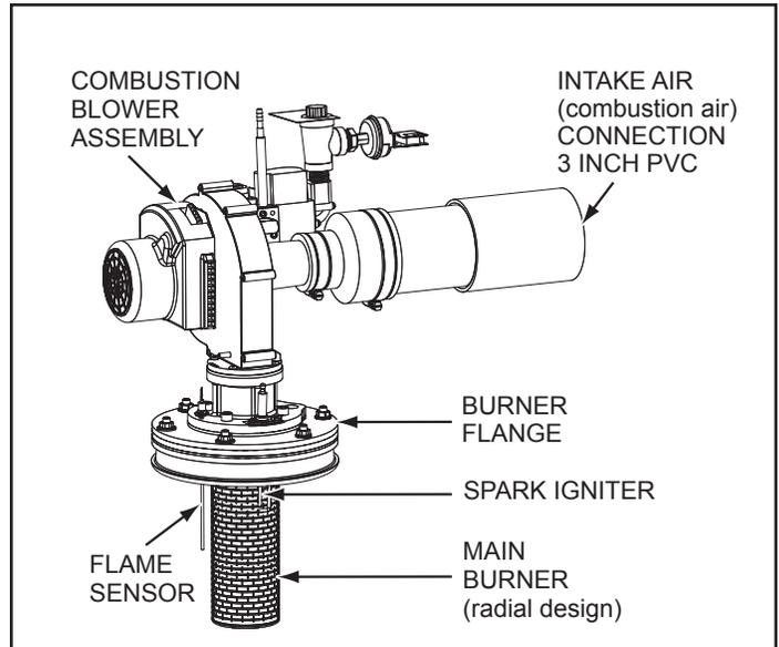
Figure 2. Blower/Burner Components
