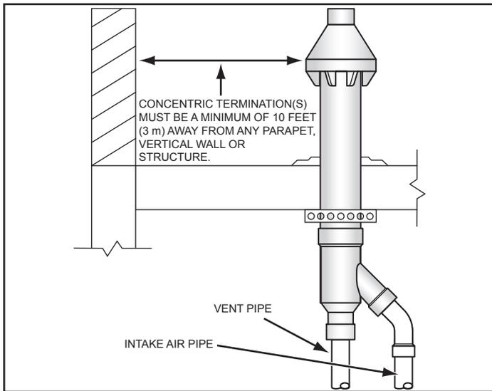
**Figure 27. Concentric Termination - Flat Roof Clearance**
