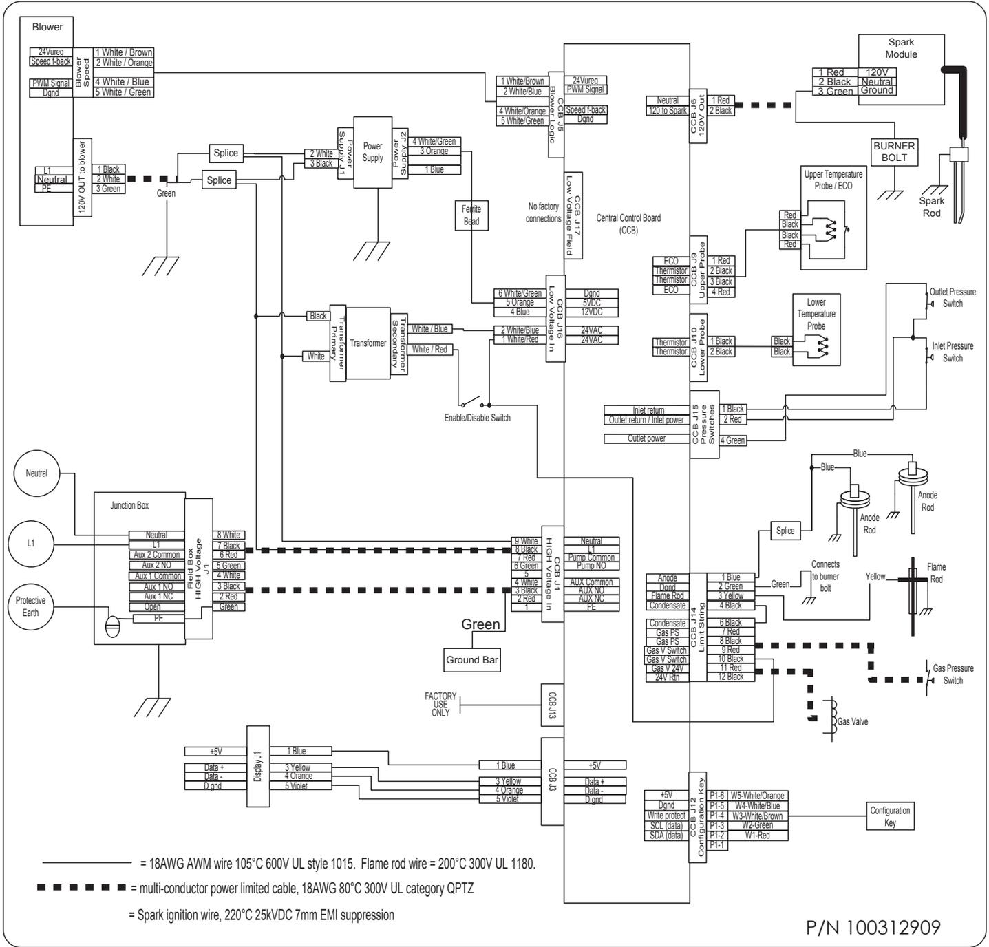
Figure 67. Wiring Diagram
