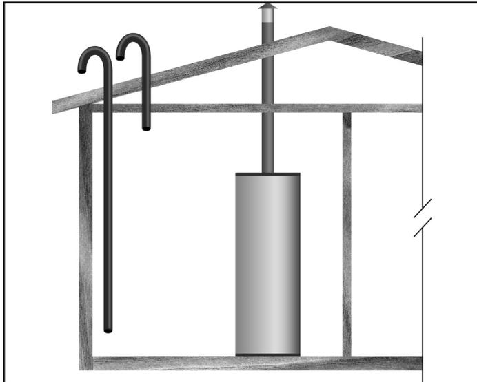
Figure 12. Two Vertical Ducts
