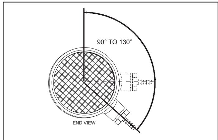
**Figure 15. Orientation of Intake Air Tee Fittings**
