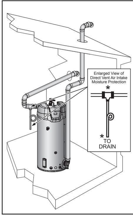
Figure 46. Direct Vent Vertical Vent Horizontal Intake
