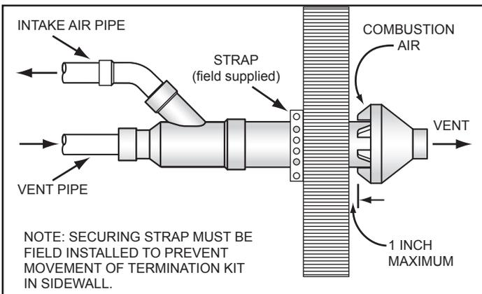
**Figure 30. Concentric Termination Clearances - Side-Wall Installation**
