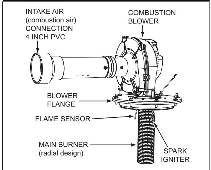
Figure 2. Blower/Burner Components
