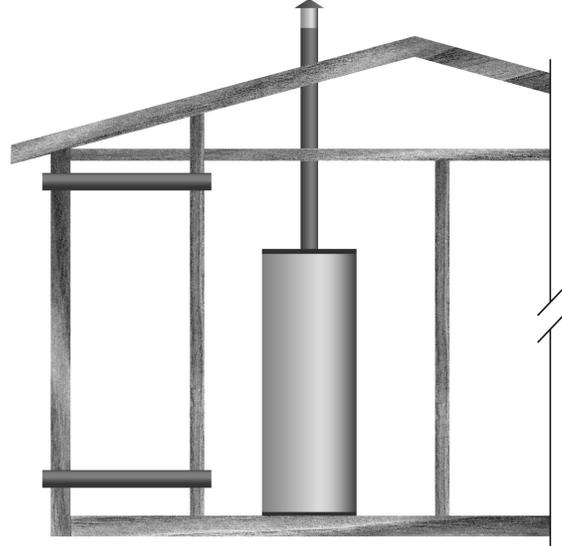
Figure 12. Outdoor Air Through Two Horizontal Ducts
