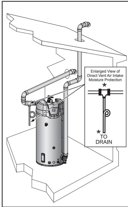
Figure 43. Direct Vent Vertical Vent Horizontal Intake
