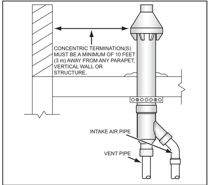
**Figure 24. Six-inch Concentric Termination - Flat Roof Clearance**
