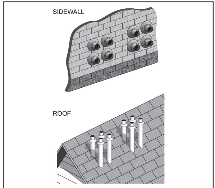
Figure 35. Eight Concentric Terminations - Sidewall and Roof
