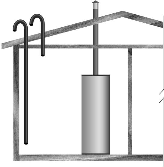
**Figure 13. Outdoor Air Through Two Vertical Ducts**
