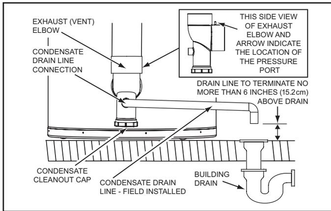
Figure 9. Exhaust/Condensate Elbow
