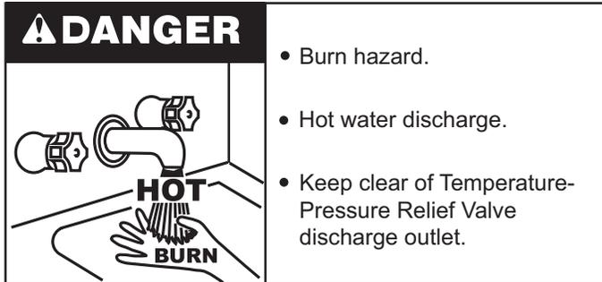
It is recommended that the Temperature-Pressure Relief Valve should be checked to ensure that it is in operating condition every 6 months.
