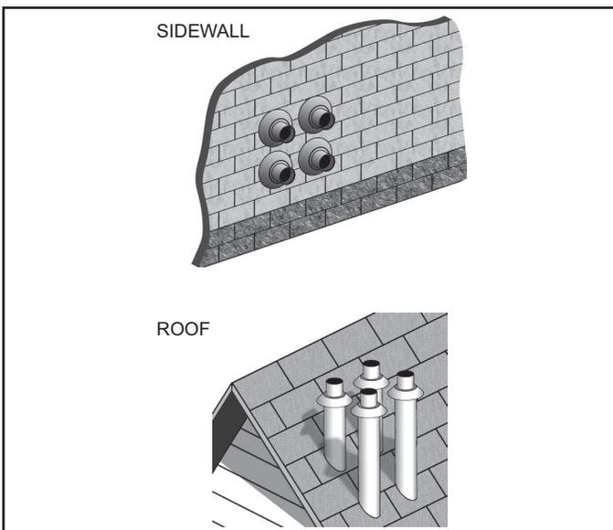
Figure 34. Four Concentric Terminations - Sidewall and Roof
