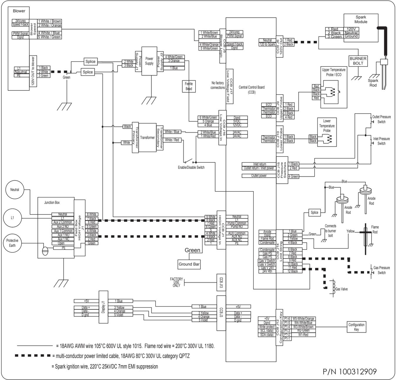
Figure 62. Wiring Diagram
