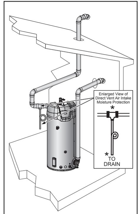
Figure 44. Direct Vent Horizontal Vent Vertical Intake
