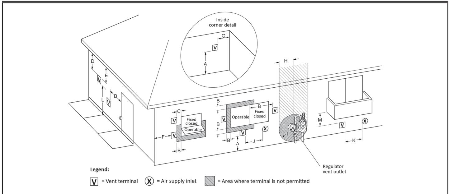
Figure 48. Sidewall Power Vent Using Outside Air
