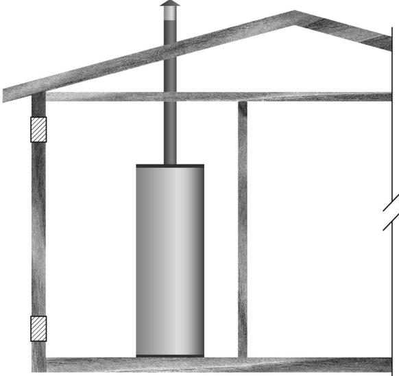
Figure 10. Outdoor Air Through Two Openings
