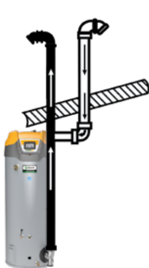
SEALED DIRECT VENT VERTICAL
