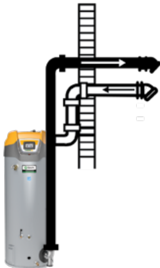
SEALED DIRECT VENT SIDEWALL
