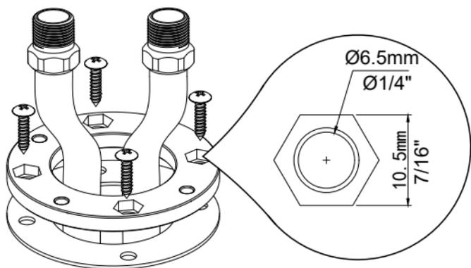
Use appropriate screws according to the surface you are fastening the floor flange to (screws not included).
