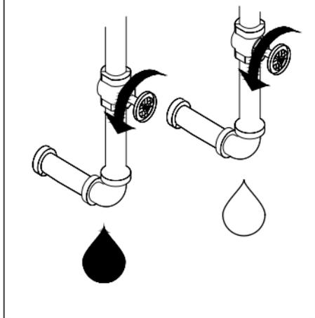
Once the welding is finished, purge the water supply system for around 30 seconds.
