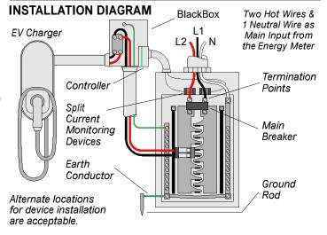
\*This device does not need additional breakers to what is required to feed the 240-208VAC end device to be controlled. The service size and end device current is to be set by the installer. See installation manual. Designed and manufactured in Canada. Inspected and labeled by Intertek in Canada.
