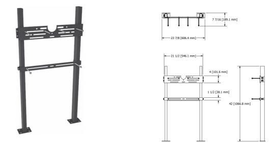
Universal floor mounted in-wall carrier designed for wall hung basins and water coolers. Steel uprights with welded feet. Includes lower bracket for added support. Mountain hardware included. Outside dimensions 7 7/16 x 23 7/8 x 42"
