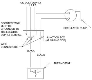
IF WIRE HAS TO BE REPLACED IN THE FIELD, USE ONLY TYPE TEW 105°C WIRE
