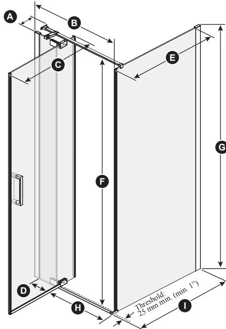
**Door dimensions****A** 129 mm (5")**B** 813 mm to 965 mm (32" to 38")**C** Mobile panel: 760 mm (29 15/16")**D** Fixed panel: 230 mm (9")**E** Return panel: 798 mm (31 7/16")**F** 1941.5 mm (76 7/16")**G** Door Height: 1956 mm (77")**H** 520 to 650 mm (20 1/2" to 25 1/2")**I** 864 mm to 883 mm (34" to 34 3/4")**J** 530 mm to 680 mm (20 7/8" to 26 3/4")**K** Min. Clearance: 190 mm (7 1/2")**L** Excess 77 mm to 229 mm (3" to 9")
