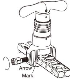
7. Turn the flare handle clockwise and continue until the clutch engages (clicking).
