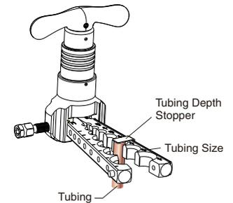
5. Close flaring bar and move the flaring body positioned over the tubing. It should click.
