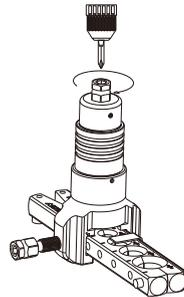
8. Reverse the direction of the drill to turn counterclockwise and start the drill until the upper position of the flaring cone is reached and the clutch engages (clicking)
