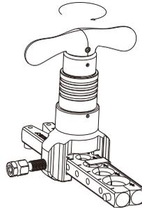
8. Turn the flare handle counterclockwise until the upper position of the flaring cone is reached and the clutch engages (clicking).
