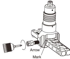
7. Using 1/4" hex drill bit, insert it to the hex socket on the expander end. With the drill set for clockwise turning, start the drill and continue until the clutch engages (clicking).
