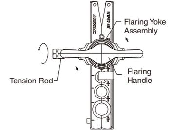
2. With the hex screws facing down on the flaring bar, open the flaring bar and insert the flaring bar into the flaring body where the arrow is pointed.
