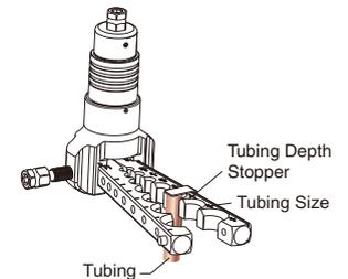
5. Close flaring bar and move the flaring body positioned over the tubing. It should click.
