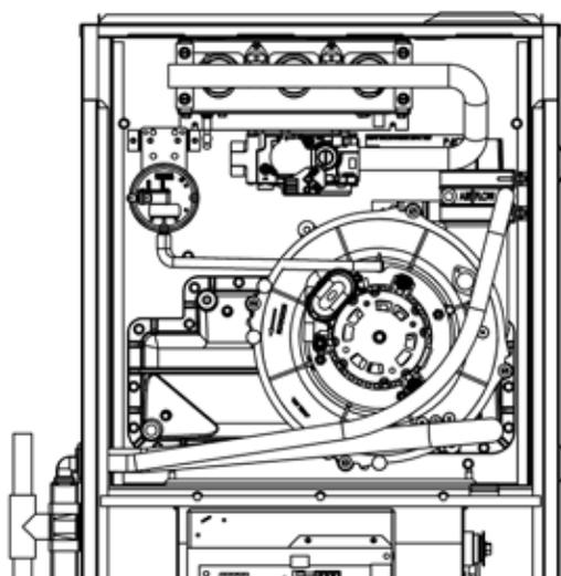
ÉVACUATION AU DESSUS - INSTALLATION DU DRAIN À GAUCHE
