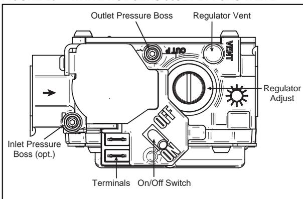
**FIGURE 29 - VALVE PRESSURE CHECK KIT**
