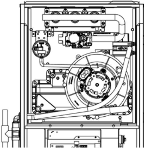
TOP VENT - LEFT DRAIN INSTALLATION (INTERNAL)
