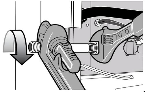
Install a manual gas shut-off valve and dirt pocket as close to the furnace as possible. Some local codes call for the manual gas shut-off valve to be located between 4 feet (1.2m) to 5 feet (1.5m) above floor level to prevent tampering by small children. Ensure that the valve is readily accessible.
