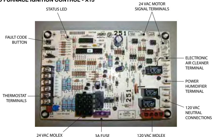
FIGURE 31 - ELECTRICAL CONNECTIONS / MOLEX CONNECTOR
