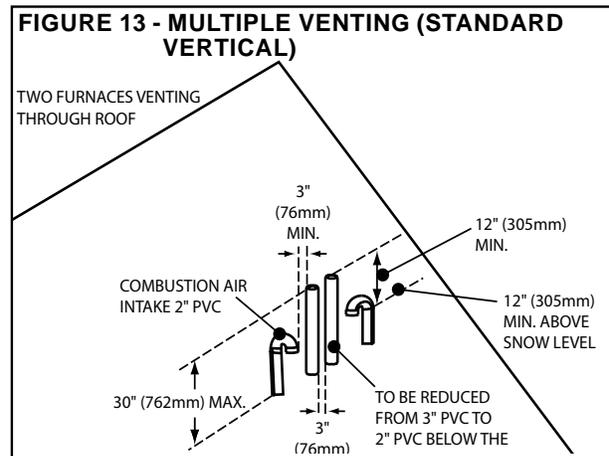
If more than two furnaces are being installed in close proximity, each additional combustion air intake and exhaust termination set shall not terminate less than 12 in (305mm) apart. Note: Canadian installations of 120000 Btu/hr require 3 ft (915mm).
