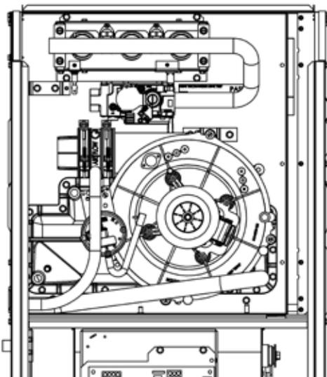
**LEFT VENT - RIGHT DRAIN INSTALLATION (INTERNAL)**
