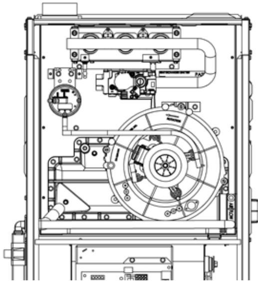
RIGHT VENT - LEFT DRAIN INSTALLATION (INTERNAL)
