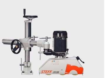
The 2038 is a professional-grade power feeder that delivers precision control on shapers, jointers, and table saws through three 4-3/4" diameter rollers across eight speeds with quick gear-lever speed changes, allowing operators to match exact feed rates to material characteristics from ultra-slow veneer work to high-volume hardwood production without compromising surface finish quality or
