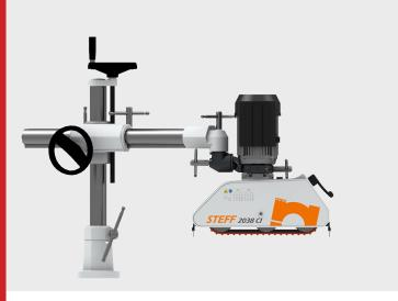
The 2038CI is a specialized belt-driven power feeder that handles short-stock and narrow workpieces on shapers, jointers, and table saws through three toothed belts across eight speeds with gear-lever speed changes, allowing operators to process small-dimension materials like picture frame stock, trim pieces, and narrow boards that would slip under traditional rollers without compromising grip, operator safety, or surface finish quality.
