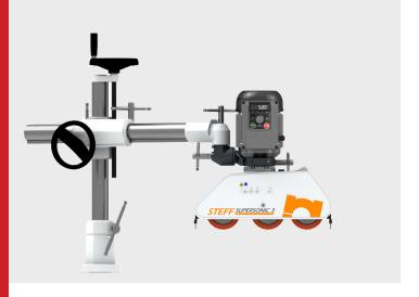
The Supersonic 3 is a professional variable-speed power feeder that provides infinite speed adjustment from 16 to 82 FPM through three 4-3/4" diameter rollers controlled by a SMART electronic controller, allowing operators to dial in precise feed rates for varying material densities and machining operations on shapers, jointers, and table saws with instant forward/reverse selection without compromising operator safety or surface finish quality.
