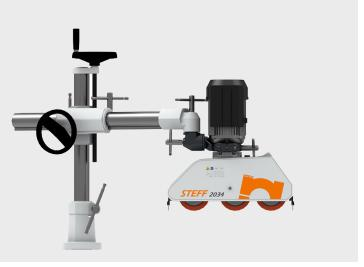
The 2034 is a professional-grade power feeder that eliminates kickback risk on shapers, jointers, and table saws by delivering consistent feed pressure through three 4-3/4" diameter rollers across four speeds, allowing operators to process everything from delicate veneered panels to high-volume production runs without compromising operator safety or surface finish quality
