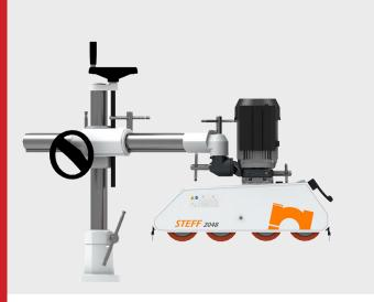
The 2048 is a professional-grade power feeder that combines maximum control with precision speed matching through four 4-3/4" diameter rollers across eight speeds with gear-lever speed changes, allowing operators to handle complex machining on medium to large workpieces from ultra-slow veneer applications to high-volume hardwood production on shapers, jointers, and table saws without compromising operator safety or surface finish quality.
