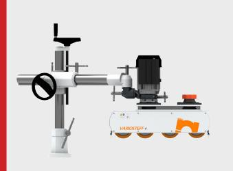
The Variostef 4 is a professional mechanical variable-speed power feeder that provides continuous speed adjustment from 10 to 59 FPM through four 4-3/4" diameter rollers controlled by a simple knob adjustment, allowing operators to adapt feed rates on the fly for varying material types and machining operations on shapers, jointers, and table saws without stopping production or compromising operator safety or surface finish quality.
