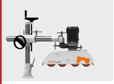
The 2044 is a professional-grade power feeder that maximizes control on medium to large workpieces through four 4-3/4" diameter rollers across four speeds (13-26-36-72 FPM), allowing operators to handle complex machining with significant material removal on shapers, jointers, and table saws by providing two infeed rollers for pulling and two outfeed rollers for holding without compromising operator safety or surface finish quality.
