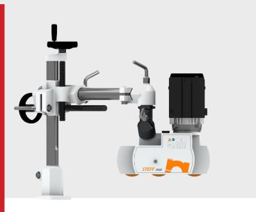
The 2032 is entry-level power feeder that transforms operations on table saws, shapers, and jointers by maintaining consistent feed pressure through three rubber rollers across four speeds, allowing operators to handle everything from delicate hardwoods to production runs without compromising safety or surface quality.
