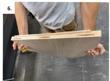
P-System slots after being machined
