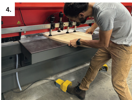
Load components onto machine and clamp down using foot pedal
