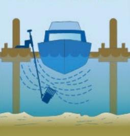
Extends up to 10 ft. from mounting bracket Mounts at an angle for maximum clearance
