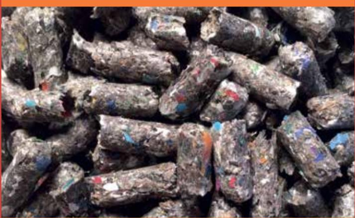
We transform shredded solid recovered fuel into Solid Improved Recovered Fuel pellets. Easily transportable by rail, road or boat and easily handleable both pneumatically and mechanically. A particle size of 2-3mm means they can be co-milled with or even completely replace coal or wood pellets to generate power, in steel and cement production, or any industry requiring high levels of heat.
