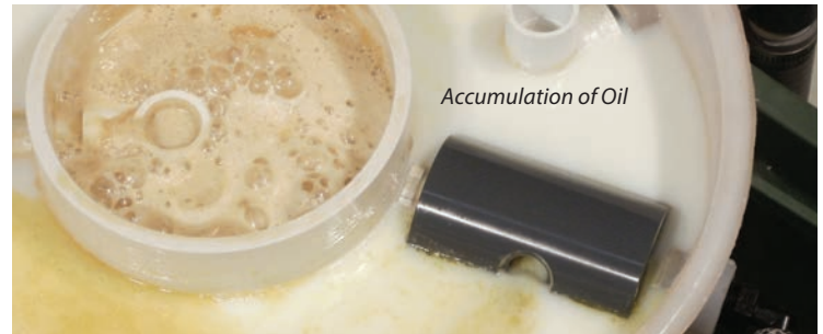
Flexor in action, with Sumpster, removing tramp oil (and a glob of biofilm), cleaning a neglected sump in under two hours.
