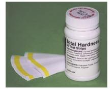
Hardness Testing Sticks 0-1000 ppm calcium carbonates anesium
