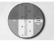
Your coolant may not measure 1:1 on the scale of this refractometer. Please correct your reading by multiplying the reading on the scale by your coolant's refractomer factor, which can be found on the coolant's product label (if there is not one listed on the label, contact your coolant supplier or manufacturer for this data).
