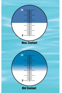
Oil emulsion is signified by the blurriness of that line. When the viewpiece is so blurry that a line is not discernible, it is time to change the coolant.
