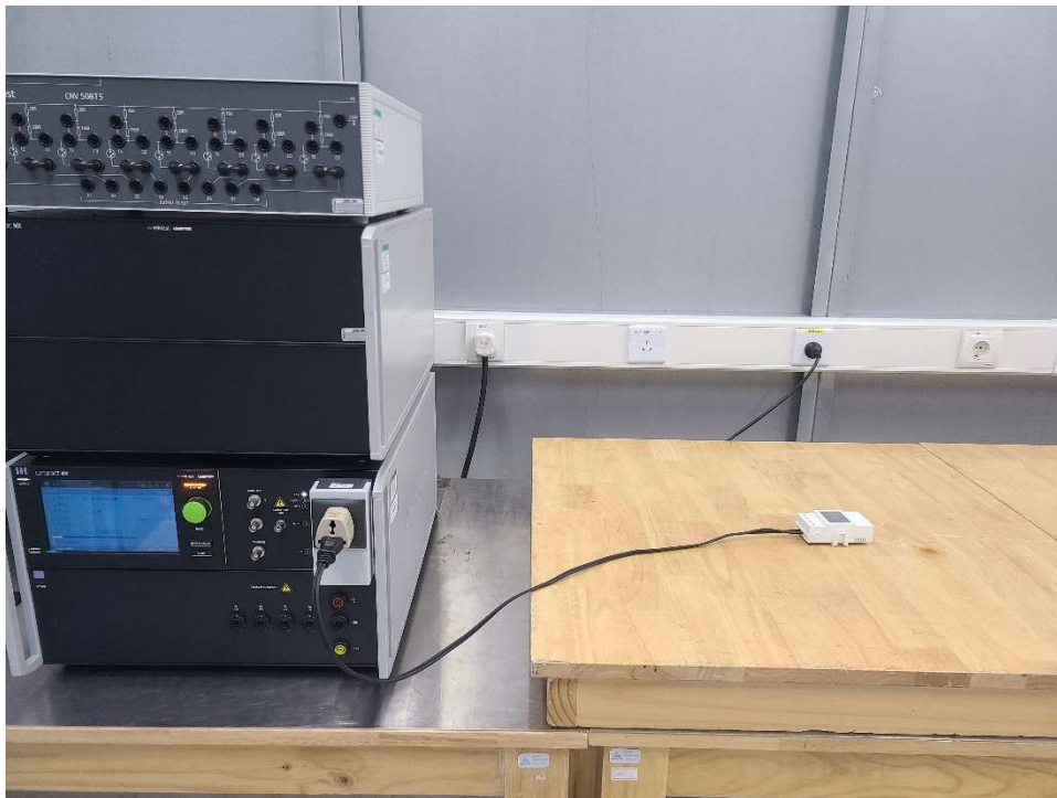
Photograph 8: Set-up for Electrical Fast Transients & Surge & Voltage Dips and Interruptions
