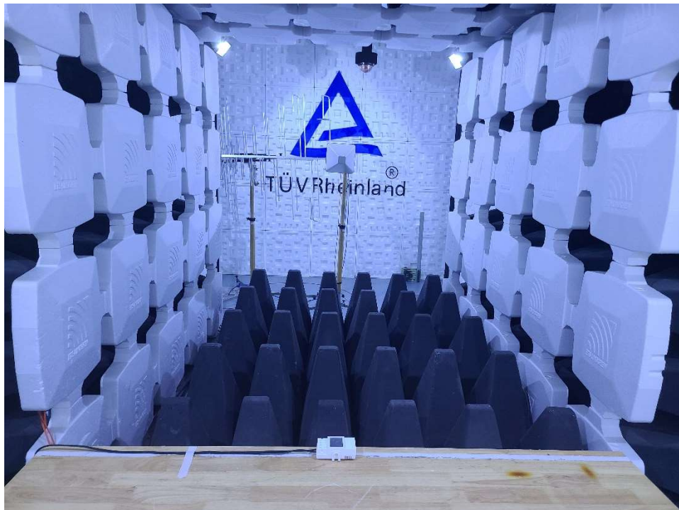
Photograph 6: Set-up for Radio Frequency Electromagnetic Field (RS), Above 1GHz
