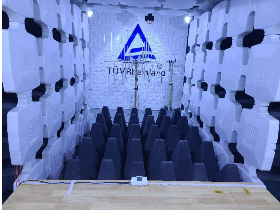
Photograph 5: Set-up for Radio Frequency Electromagnetic Field (RS), Below 1GHz
