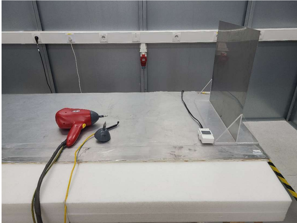
Photograph 7: Set-up for Electrostatic Discharge (ESD)
